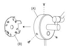
Attach the lamp body back to the wall mounting.
