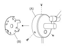
Remove the wall mounting (B) by unscrewing three screws from the lamp body (A).
