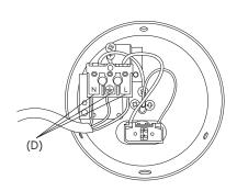
4. Connect the electrical cord with the terminal strip.
