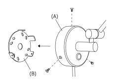
Remove the wall mounting (B) by unscrewing three screws from the lamp body (A).
