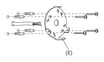
3. Position the wall mounting making sure the metal handle (E) is covering the hole on the lamp body. Mount it with four appropriate screws and plugs. Always use correct screws and plugs for the mounting surface.
