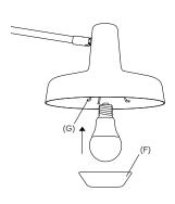
6. To insert the light bulb, release the undershade (F) by pressing three undershade brackets (G) inwards.
